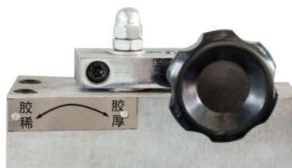
Figure 8 Glue quantity regulating handle
